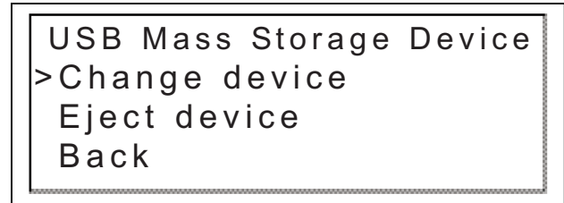
Fig 10.1 - Pressing Shift+Power to access the Device Menu
