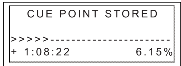
Fig 9.2 - Cue Point Memorization using Shift+Cue
